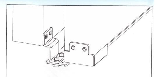
8 At the bottom, connect the two panels together with bolt
