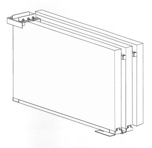
12 Install the bracket and the assembly is complete
